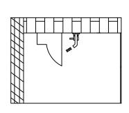
4) Connect inside pipe and test for leak checking
